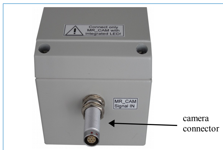
Figure 2: Filter box (front side)
