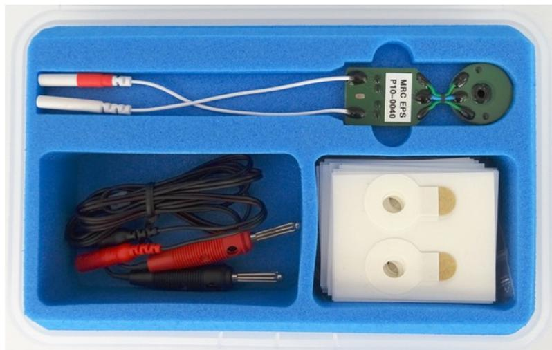
Figure 6: HFS electrode and accessories placed in the storage box
