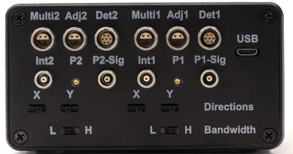
Figure 4: Side panel of the Compact controller with additional "Adjust-In" inputs for electronic adjustment of the x and y positions on the PSD detectors.
