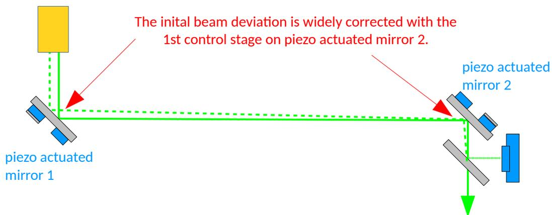
Figure 2: The principle of correcting a position error
